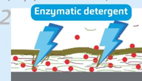
In order to remove biofilm, the EPS matrix, the shield of the biofilm has to be destroyed with an enzymatic detergent.
